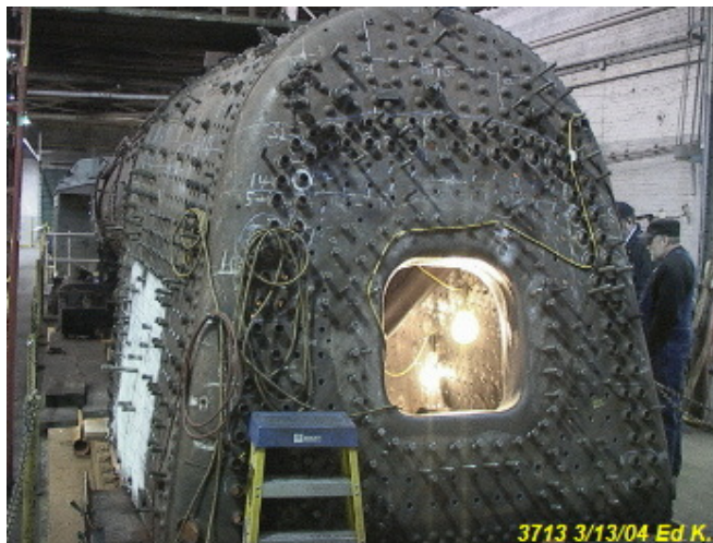
Veiw of locomotive showing staybolts
